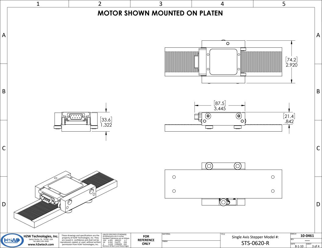
1 LINEAR STEPPER MOTOR SPECIFICATIONS STS-0620-R Motor P/N Continuous Force 6.0 lbs 26.7 N **Rated Current** 2.0 Amp Resistance/Phase @ 20C 2.40 ohms Inductance/Phase @ 20C 3.0 mH **Motor Phases Bearing Type** Roller Bearing Nominal Airgap 0.0015" **Motor Mass** 9.8 oz 279 grams Platen Mass 5.0 g/mm 0.28 lbs/in
